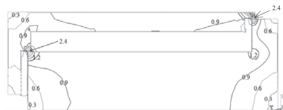
Fig. 5 Contour graph of magnetic flux density (Unit [T]) ( s = 3.0 \text{ mm} , x = 2.0 \text{ mm} , NI = 1,106 \text{ AT} )
