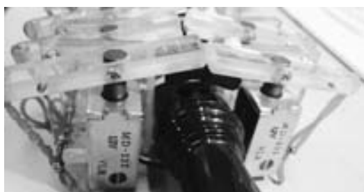
Fig. 2 Fingering part (solenoid plungers)
